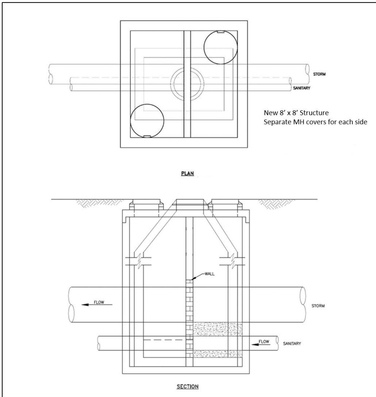
The following assumptions were used to develop the unit cost for replacing existing dividing wall manholes with new structures to separate the existing storm and sanitary sewers.
