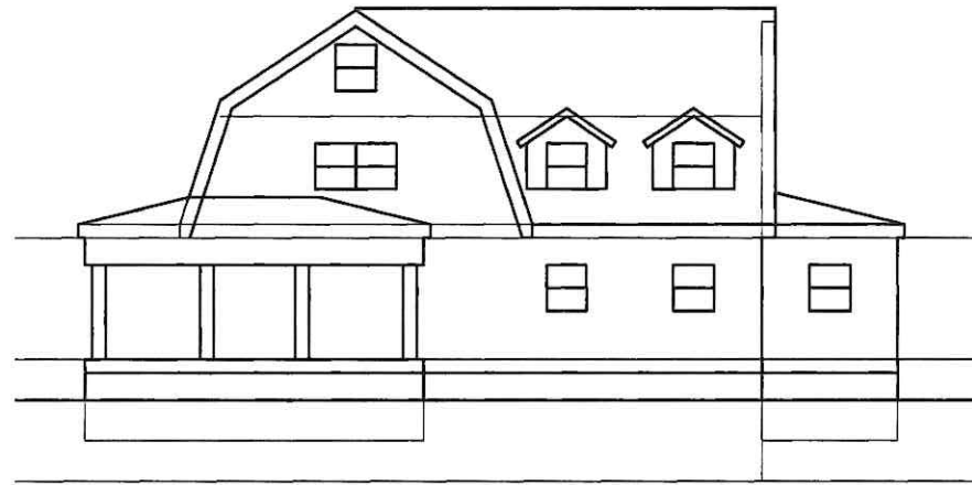
1 Proposed North Elevation A4 Scale: 1/16" = 1'-0"
