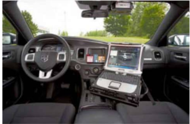
Example of vehicle-installed ALPR system enforcement devices
