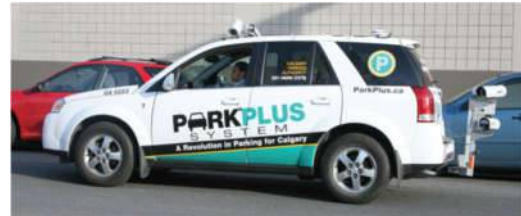
Example of vehicle equipped with ALPR enforcement cameras
